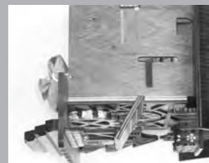
Try the clock by moving the minute (long) hand to the next half/full hour and see whether the cuckoo calls. If that does not help immediately, try to move the bar several times up and down (in and out), and move the minute hand on the next half/full hour
