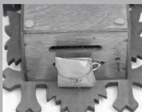
3. The night-off handle may not be in the correct position. The clock has a manual night-off handle. It is either underneath the cuckoo clock cabinet (shaped like a ring) next to the hook of the left weight or at the left wall (shaped like a bar). If you move this up (push it), you can turn the cuckoo off. If you move it down (pull it), the cuckoo calls on the half hour and on the hour.
