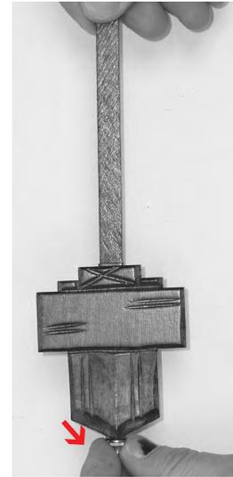
Some of our have a screw pendulum. The speed of the clock is regulated by the length of the pendulum. The pendulum length can be changed by turning the adjustment nut on the bottom of the pendulum.
